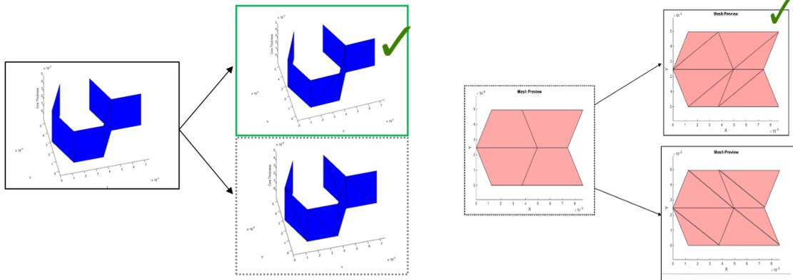
(a) Core hexagonal cell mesh triangularization (b) Face cell mesh quadrangulization
