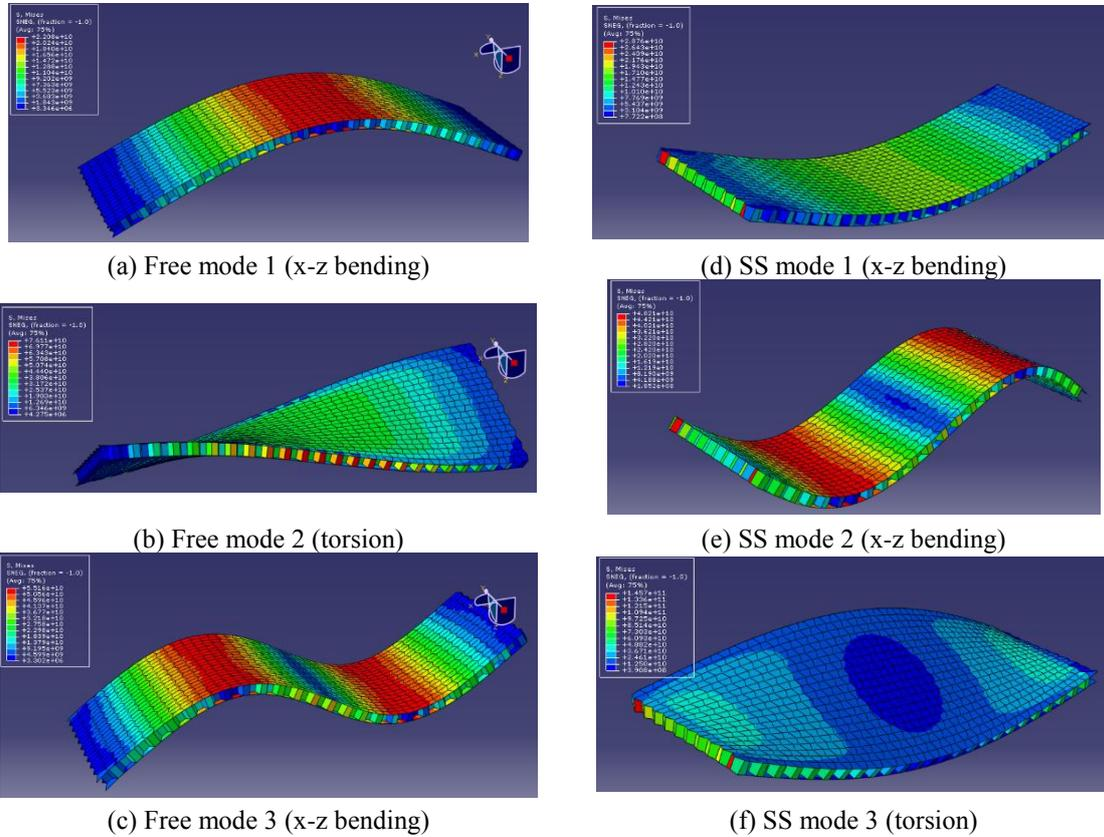
Fig. 8 Hexagonal honeycomb sandwich panel simulated first 3 modes for free (left) and SS (right) BCs
