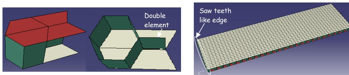
(a) Hexagonal honeycomb core mesh basic cell (b) Detailed FE 3D mesh of the sandwich panel
