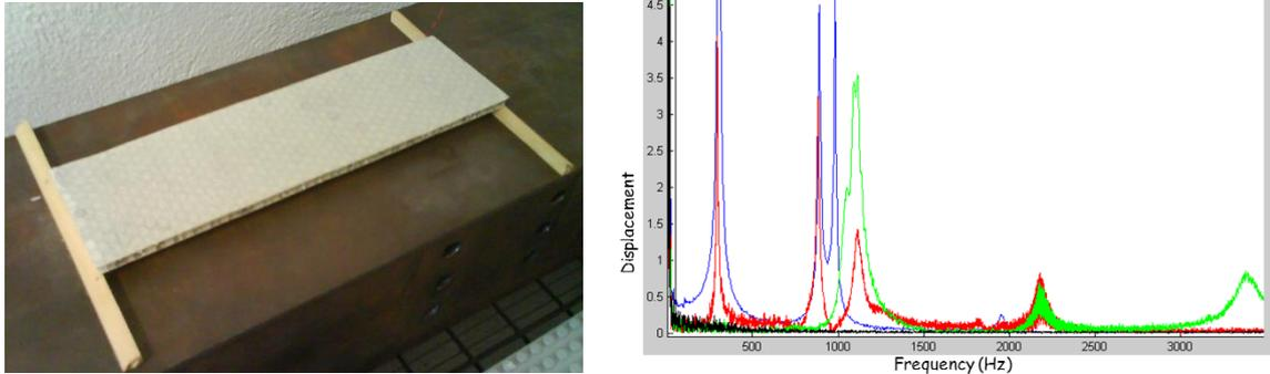
(a) Honeycomb sandwich panel SS configuration (b) FTF frequency responses (colors indicate measurements at different points as in Fig. 4a)
