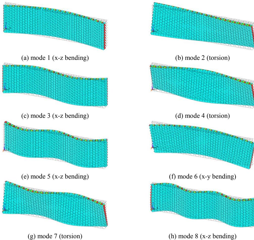
Fig. 13 Hexagonal honeycomb sandwich panel simulated first 8 modes under free BCs using ANSYS2
