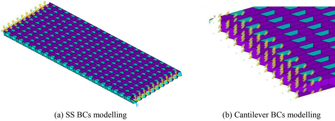
Fig. 11 Implementation for ANSYS® of the SS and cantilever BCs using the detailed FE 3D approach
