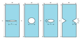
Fig. 2 Plate with different notch geometry, thickness of 2 mm and the applied tensile displacement U of 2 mm
