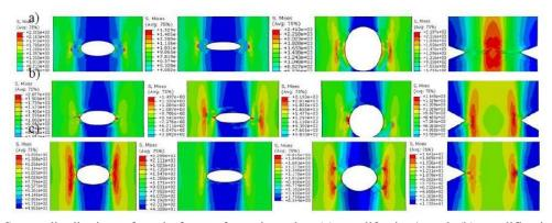
Fig. 6 Stress distribution of each form of notch under (a) modification1 and (b) modification 2 (c) modification3
