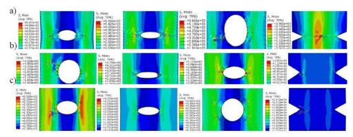
Fig. 9 Stress distribution of each form of notch under (a) modification1 and (b) modification 2 (c) modification3
