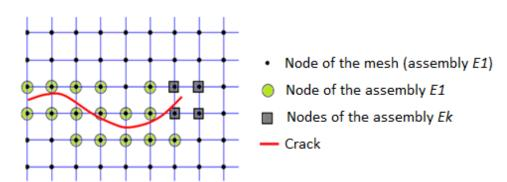
Fig. 1 Description of the E1EJEK sets of the displacement field approximation enriched finite element
