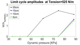
Fig. 12 Limit cycle amplitudes as a function of dynamic pressure: pre-tensioned
