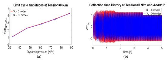
Fig. 5 (a) Limit cycle amplitudes as a function of dynamic pressure untensioned and (b) deflection time history at x/a, x/b=0.8,0.5, AoA=10°, untensioned
