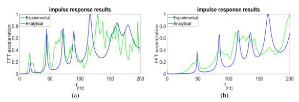
Fig. 4 Non-linear impulse response comparison: (a) Untensioned, and (b) pre-tensioned
