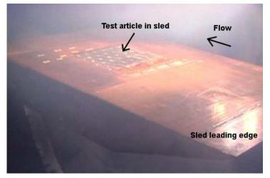
Fig. 3 TPS sample mounted in the 8' HTT sled at 5° angle of attack (Goldman et al. 2014)
