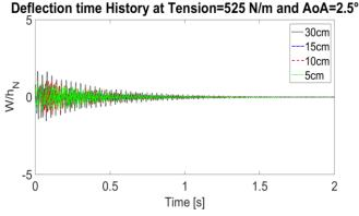
Fig. 13 Deflection time history comparison at x/a, x/b=0.8,0.5, AoA=2.5°, pre-tensioned
