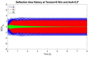
Fig. 7 Deflection time history comparison at x/a, x/b=0.8,0.5, AoA=2.5°, untensioned
