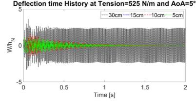
Fig. 14 Deflection time history comparison at x/a, x/b=0.8,0.5, AoA=5°, pre-tensioned
