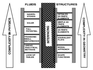
Fig. 1 Fluid and structure solvers for aero-elastic simulation for a closely coupled model (Guruswamy 2002)
