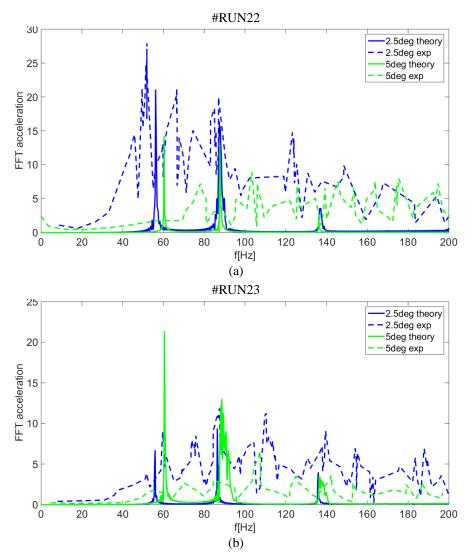
Fig. 6 Non-linear response comparison between experiment and theory for #RUN22 (a) and #RUN23 (b) at x/a, x/b=0.8,0.5
