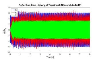
Fig. 8 Deflection time history comparison at x/a, x/b=0.8,0.5, AoA=10°, untensioned
