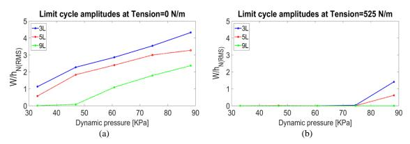
Fig. 10 Limit cycle amplitudes as a function of dynamic pressure untensioned (a) and tensioned (b)
