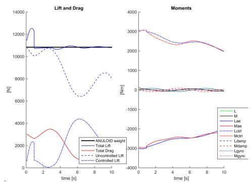
Fig. 12 Decomposition of forces and moments during sine shaped reference on the pitch rate
