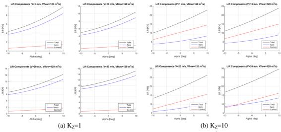
Fig. 10 Lift force components for a volume flow of  $120 \text{ m}^3/\text{s}$
