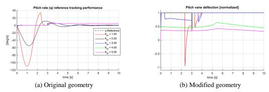
Fig. 3 Pitch rate tracking performance of the aircraft with 5 different values for  $K_M$  given a +5 deg/s pitch rate reference at 30 m/s. This figure shows that  $K_M > 3$  to prevent pitch control vane saturation. Note that for  $K_M < 3$  the aircraft is not capable at all of tracking the reference
