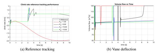
Fig. 8 Climb rate tracking performance of the aircraft with 5 different values for  $K_Z$  given a 1 m/s climb rate reference at 30 m/s. If  $K_Z >= 10$  the volume flow does not saturate beyond the transient
