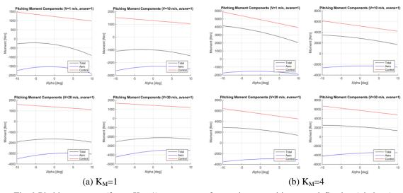
Fig. 9 Pitching moment (factor K<sub>M</sub>=1) components for maximum positive vane deflection (pitch up)
