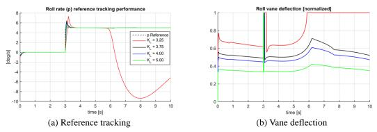
Fig. 6 Roll rate tracking performance of the aircraft with 5 different values for  $K_L$  given a 5 deg/s pitch rate reference at 30m/s. If  $K_L >= 3.75$  the pitch control vanes do not saturate for a positive pitch rate reference
