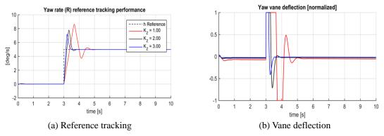
Fig. 7 Yaw rate tracking performance of the aircraft with 3 different values for  $K_N$  given a 5 deg/s yaw rate reference at 10 m/s. If  $K_N=1$  the yaw control vanes do not saturate beyond the initial transients
