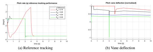
Fig. 5 Pitch rate tracking performance of the aircraft with 5 different values for  $K_M$  given a -5 deg/s (negative) pitch rate reference. If  $K_M >=3$  the pitch control vanes do not saturate for a negative pitch rate reference beyond the initial transient
