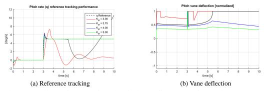
Fig. 4 Pitch rate tracking performance of the aircraft with 5 different values for  $K_M$  given a +5 deg/s pitch rate reference at 30m/s. If  $K_M >=4$  the pitch control vanes do not saturate after the initial transient for a positive pitch rate reference
