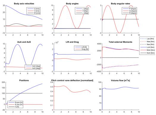
Fig. 11 Aircraft states as function of time for a sine shaped reference on the pitch rate
