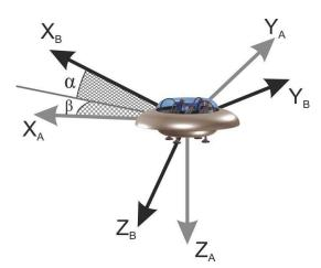
Fig. 2 Standard aircraft axis definition. Note that the  $Z_B$  axis points downwards
