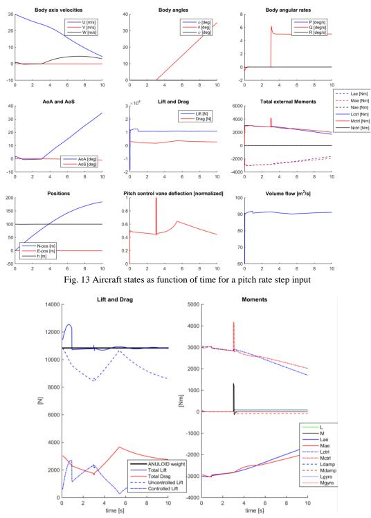
Fig. 14 Dynamic forces and moments acting on the aircraft during a pitch rate tracking task, where a pitch rate of 5 deg/s is tracked after 3 seconds. Notice the sharp peak in the resultant pitching moment during onset of the pitch maneuver
