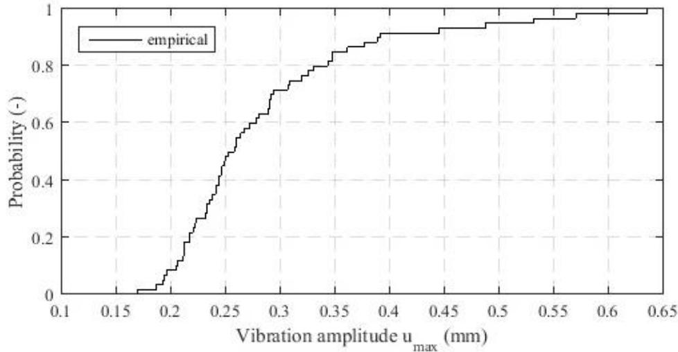
Fig. 9 Variance in maximum vibration amplitudes caused by variable material parameters
