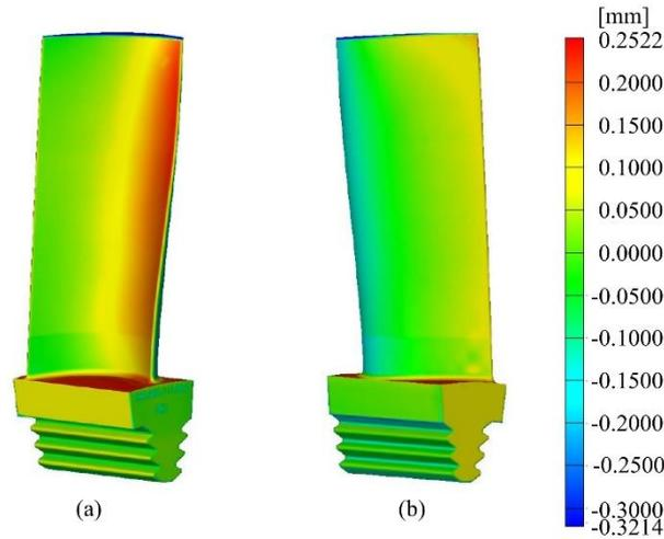
Fig. 1 Evaluated deviations between measured and ideal geometry of one turbine blade using GOM Inspect viewed (a) from the front and (b) from the back
