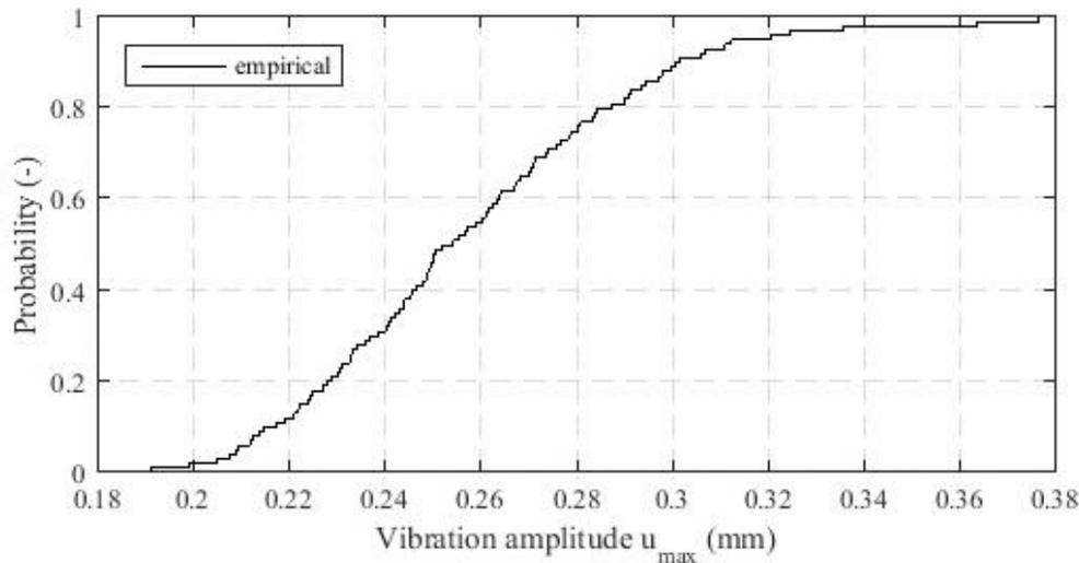
Fig. 10 Variance in maximum vibration amplitudes caused by variable material parameters of the patch
