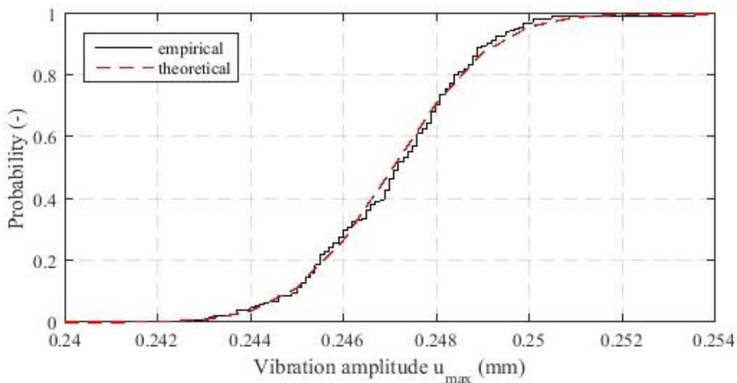
Fig. 8 Variance in maximum vibration amplitudes caused by variable geometrical parameters
