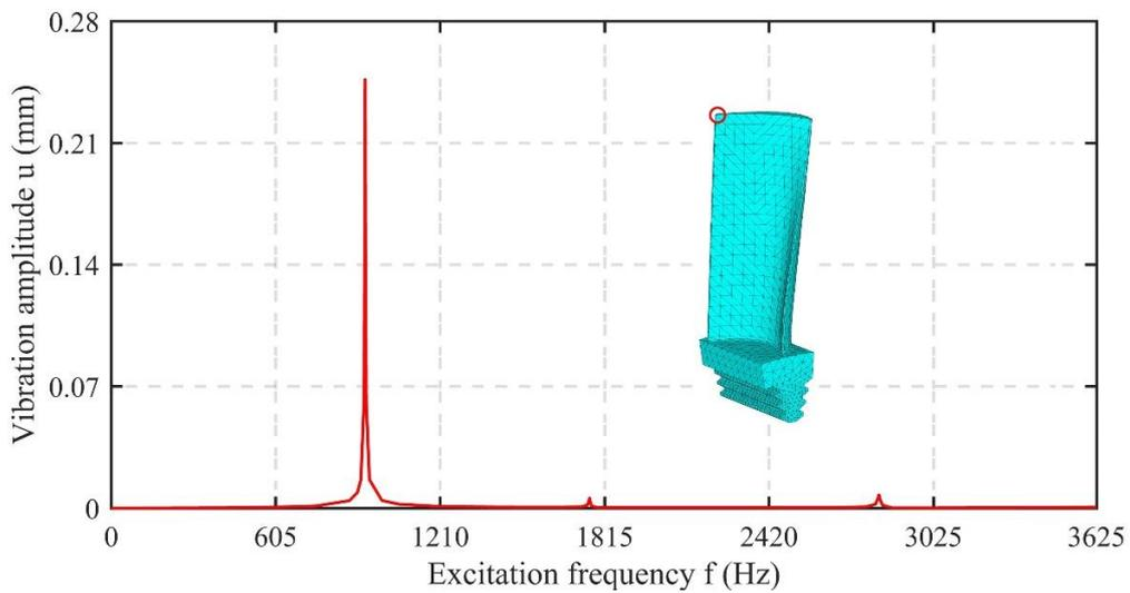
Fig. 6 Frequency response analysis of the rotor blades investigated
