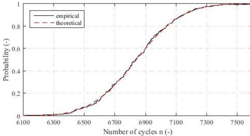
Fig. 13 Variance in lifetime caused by variable geometrical parameters
