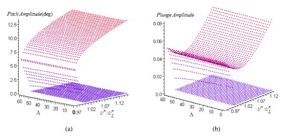
Fig. 5 Subcritical and Supercritical knee-like Hopf bifurcation diagram against wing sweep angle (a), (b) pitch and plunge amplitude
