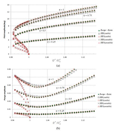
Fig. 3 finite limited amplitude of the stable and unstable LCOs for different wing sections (a) pitch amplitude (b) plunge amplitude (c) frequency
