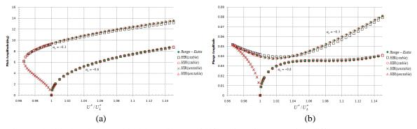
Fig. 4 Subcritical and Supercritical knee-like Hopf bifurcation diagram against different parameters (a), (b), (c), (d) pitch and plunge amplitude vs. different value of  $a_h$  (c), (d) pitch and plunge amplitude vs. different value of  $\mu$
