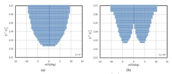
Fig. 8 Bifurcation locations for different values of  $\alpha(0)$  and  $U^*/U_L^*$  for (a)  $\Lambda=0$  (b)  $\Lambda=30^\circ$
