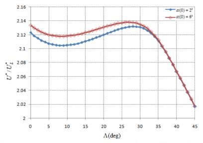
Fig. 6 Bifurcation onset location against wing sweep angle for two different initial conditions
