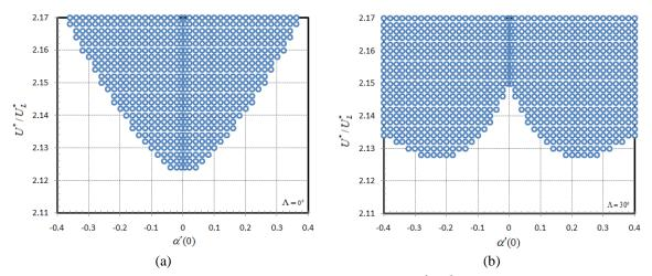
Fig. 9 Bifurcation locations for different values of  $\alpha'(0)$  and  $U^*/U_L^*$  for (a)  $\Lambda=0$  (b)  $\Lambda=30^\circ$
