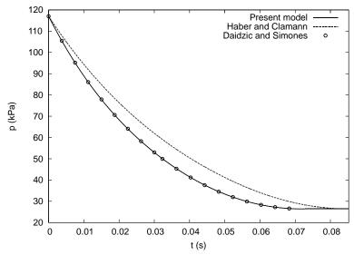
Fig. 5 Pressure history within the single chamber for V/A=10 m
