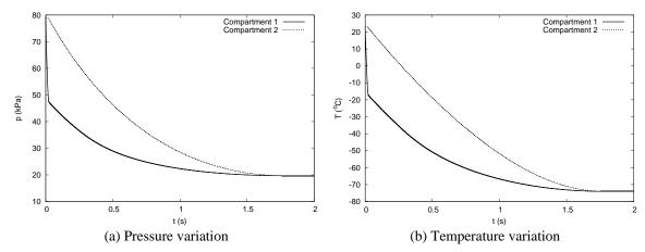
Fig. 11 Decompression of the two-compartment aircraft with translational blowout panel between compartments  $1\ \mathrm{and}\ 2$
