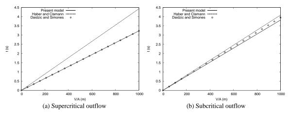
Fig. 4 Supercritical and subcritical phases durations of the single chamber for various V/A ratios
