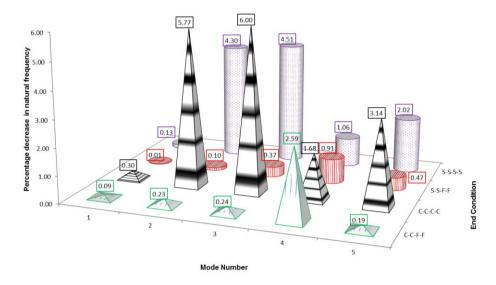
Fig. 7 Comparison of the shift in natural frequency for the four end conditions
