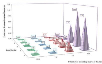
Fig. 6 Shift in natural frequency for one way simply supported panel: delamination position 2
