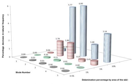
Fig. 3 Shift in natural frequency for two way clamped panel: delamination position 3
