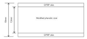
Fig. 1 Cross-sectional view of the single layer GFRP composite sandwich used for validation
