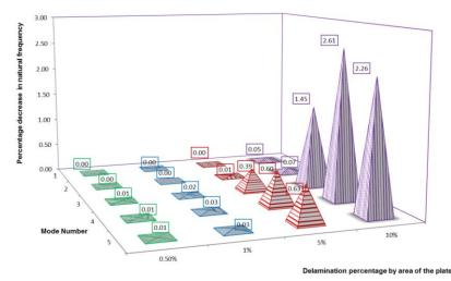
Fig. 5 Shift in natural frequency for one way clamped panel: delamination position 2
