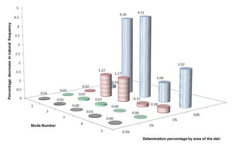
Fig. 4 Shift in natural frequency for two way simply supported panel: delamination position 3
