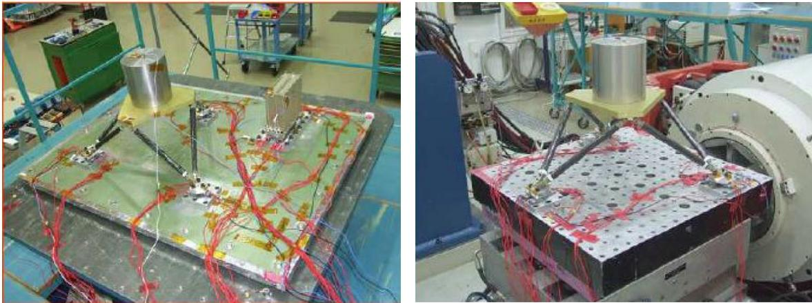
Fig. 2 IFLV total and MIRI test setup on shaker slip table, courtesy (Destefanis *et al.* 2009)
