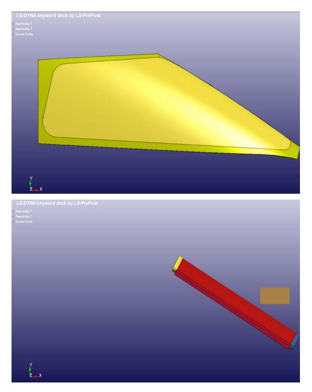
Fig. 9 Full-scale and simplified windshield models
