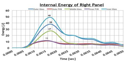
Fig. 14 Internal energy for each layer of right panel
