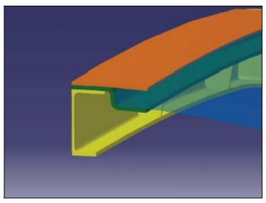
Fig. 4 Windshield-surround installation - geometry
