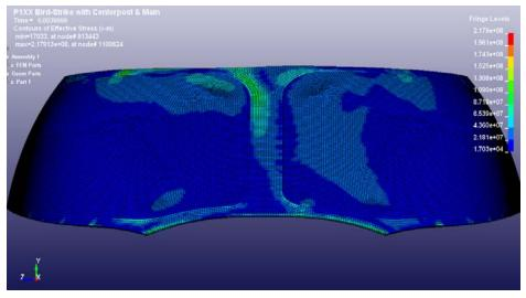
t = 0.004 sec Fig. 12 Von Mises stress on the complete windshield model
