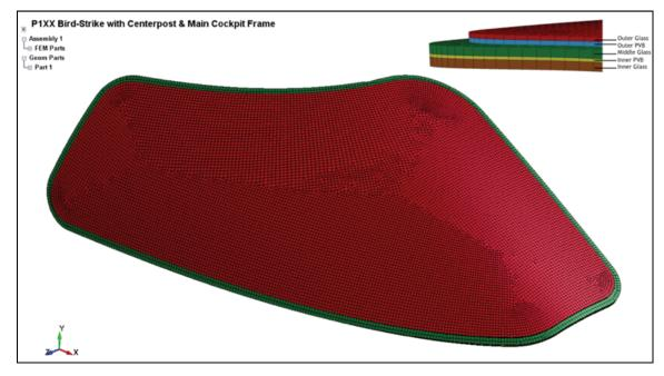
Fig. 5 Full-scale left windshield FE model
