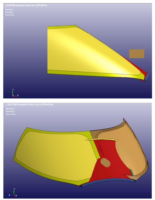
Fig. 10 Overlap of the complete and simplified windshield models
