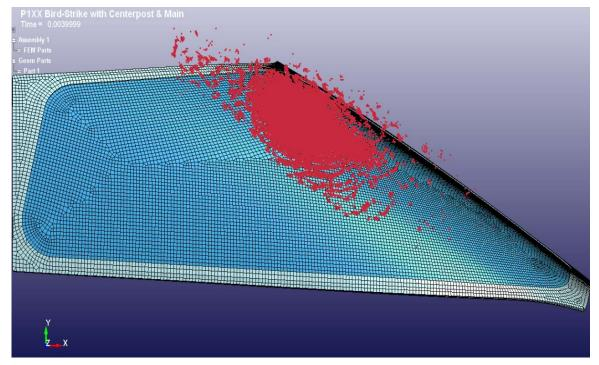
t = 0.004 sec Fig. 11 Bird impact scenario for the complete model
