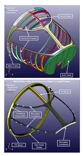
Fig. 8 Geometry and FEM of the cockpit structure
