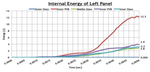
Fig. 15 Internal energy for each layer of left panel
