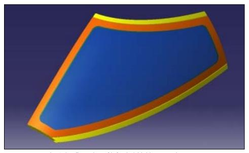
Fig. 1 Configuration of left windshield-surround structure
