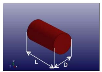
Fig. 2 Cylindrical bird model
