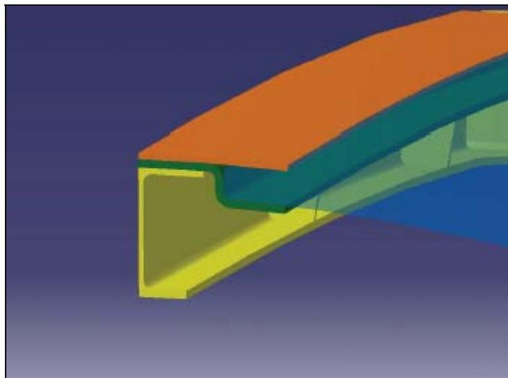
Fig. 4 Windshield-surround installation - geometry
