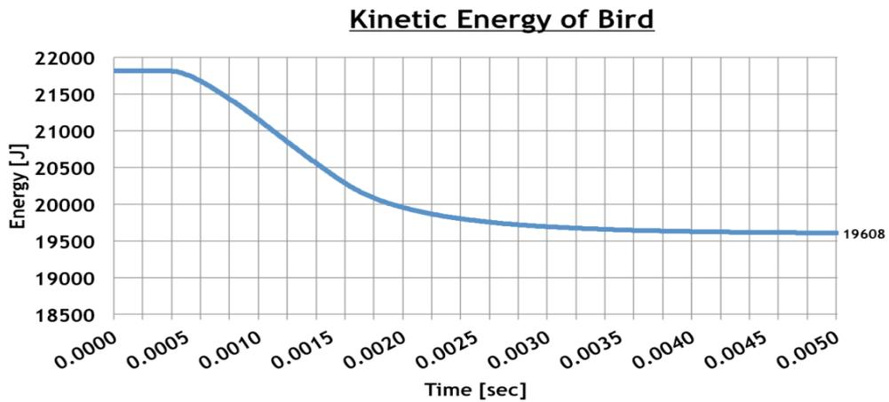
Fig. 18 Kinetic energy of the bird
