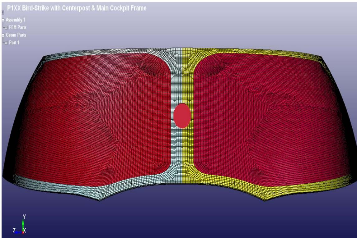
Fig. 16 Birdstrike against the center beam of the surround structure
