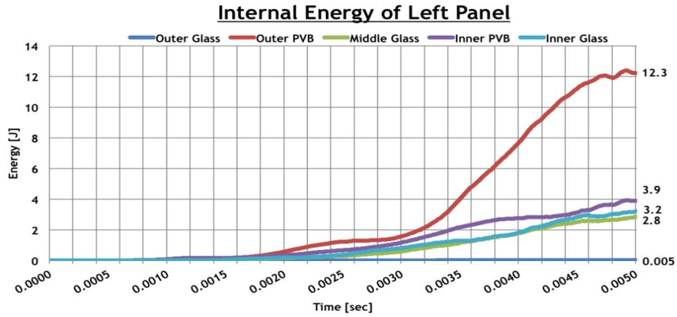
Fig. 15 Internal energy for each layer of left panel
