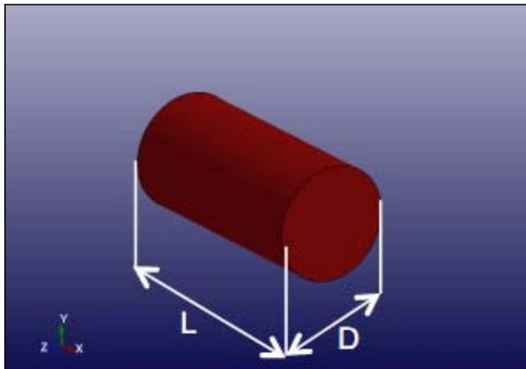
Fig. 2 Cylindrical bird model
