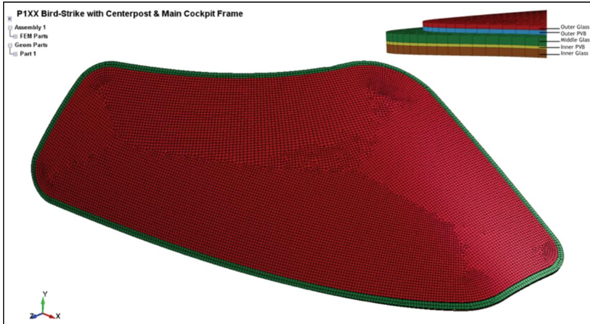
Fig. 5 Full-scale left windshield FE model
