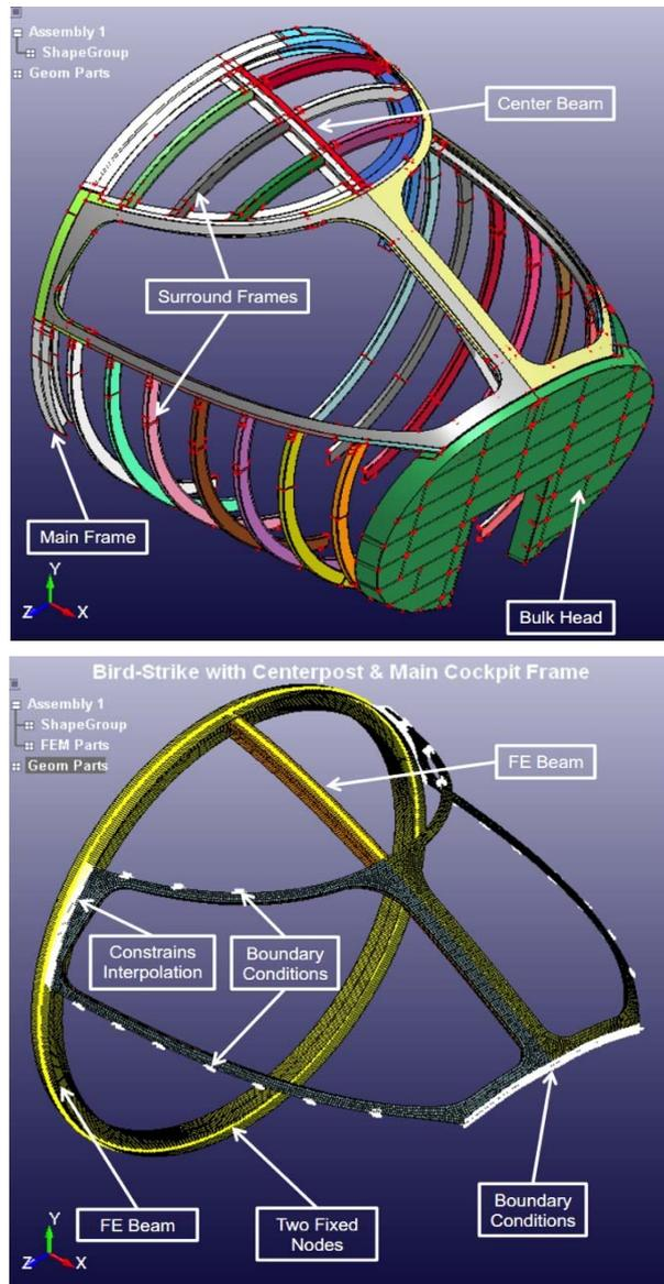
Fig. 8 Geometry and FEM of the cockpit structure
