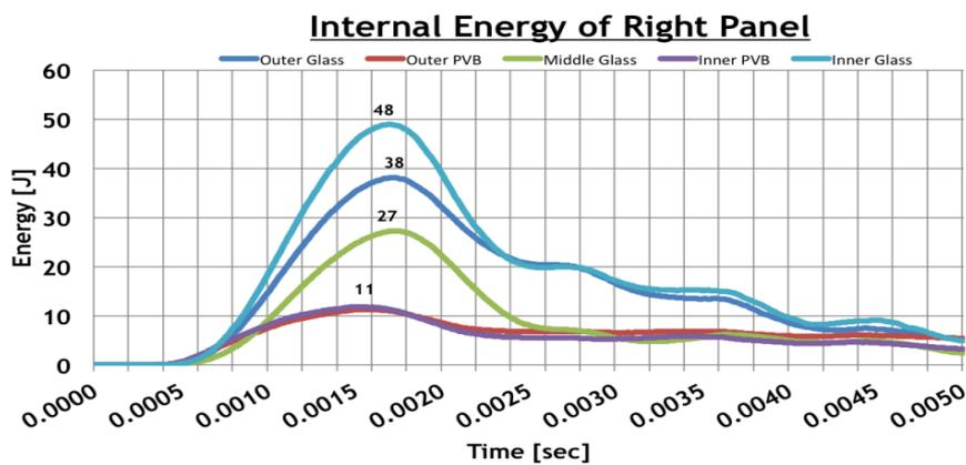
Fig. 14 Internal energy for each layer of right panel
