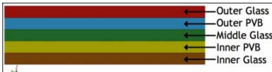
Fig. 3 Windshield lay-up configuration
