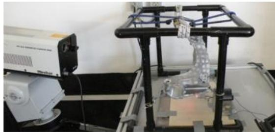
Fig. 10 Experimental set up for steering knuckle
