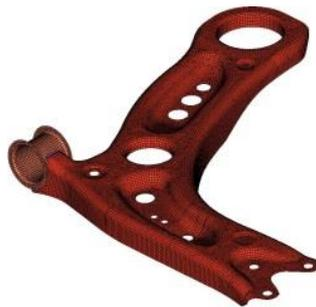
Fig. 13 FE model of the track control arm
