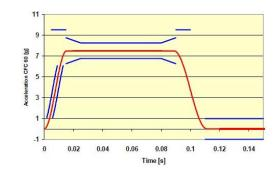
Fig. 10 High severity pulse of the euro NCAP whiplash test protocol
