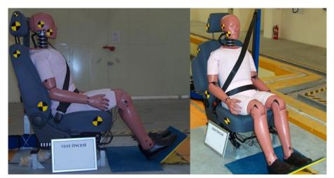
Fig. 7 Positioned dummy in the seat
