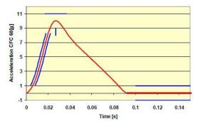
Fig. 9 Medium severity pulse of the euro NCAP whiplash test protocol
