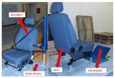
Fig. 4 Test sample elements
