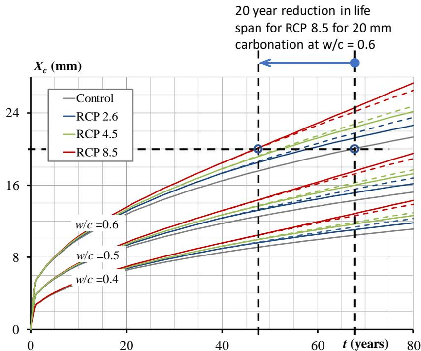
**Fig. 3** Time-dependent carbonation depth of RC structures in Sydney for the considered  $w/c$  ratios and climate change scenarios.
