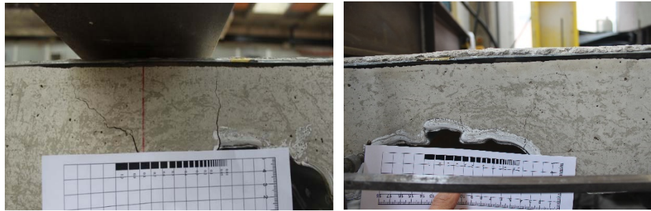
Fig. 13 Concrete cracking at and between loading points (B1b)
