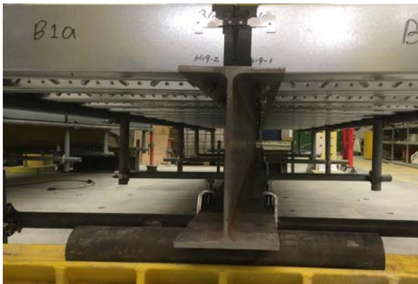
Fig. 2 Temporary supports attached to the beam
