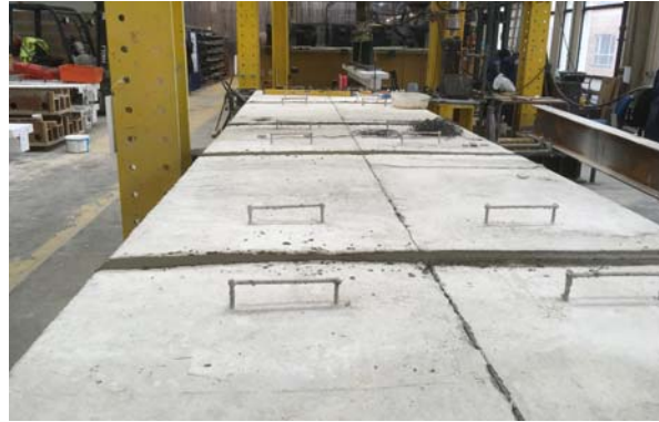
Fig. 1 Reassembled/reused slab segments with grout joints (specimen B1a REUSE)
