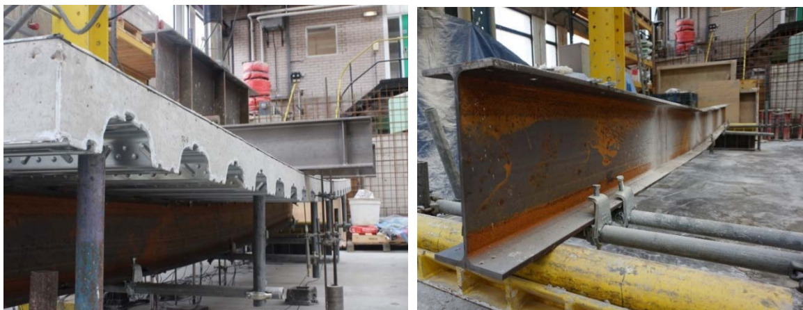
Fig. 14 Deflection of beam and slab and yielding of beam section (B1b)
