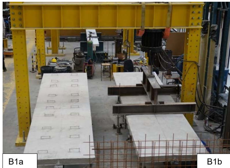
Fig. 5 Specimens after the concrete was cast
