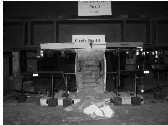
Fig. 22 Web rupture in specimen 3
