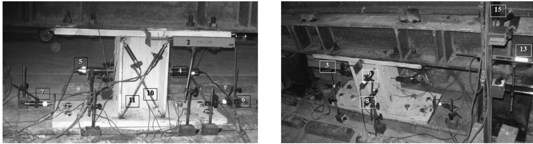
Fig. 14 Location of LVDTs on all specimens
