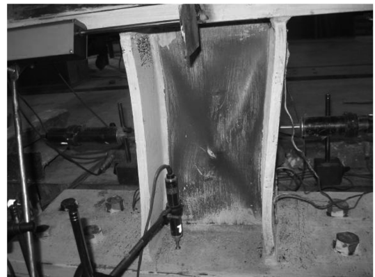
Fig. 16 Web rupture in specimen 1
